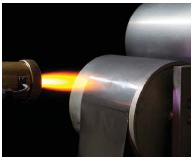
Fig. 1 – Roll-to-roll deposition process
