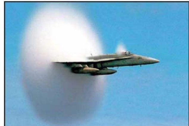
A cloud builds up around an F/A-18C Hornet as it breaks through the sound barrier above the Pacific Ocean.
